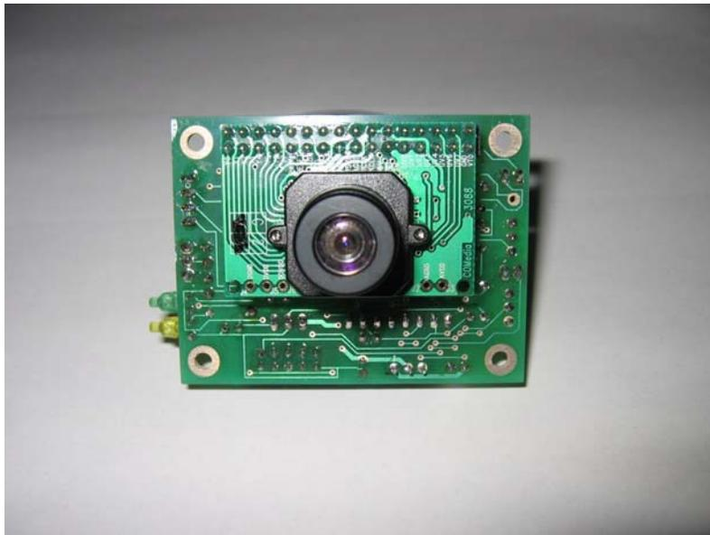
Photo 1: Front view of the AVRcam v1.1
